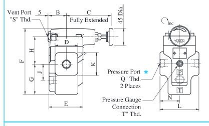
★ There are two threaded connection pressure ports. They can be connected each other in-line: one as inlet and the other as an outlet or the valve can be used by plugging one of the pressure port.
